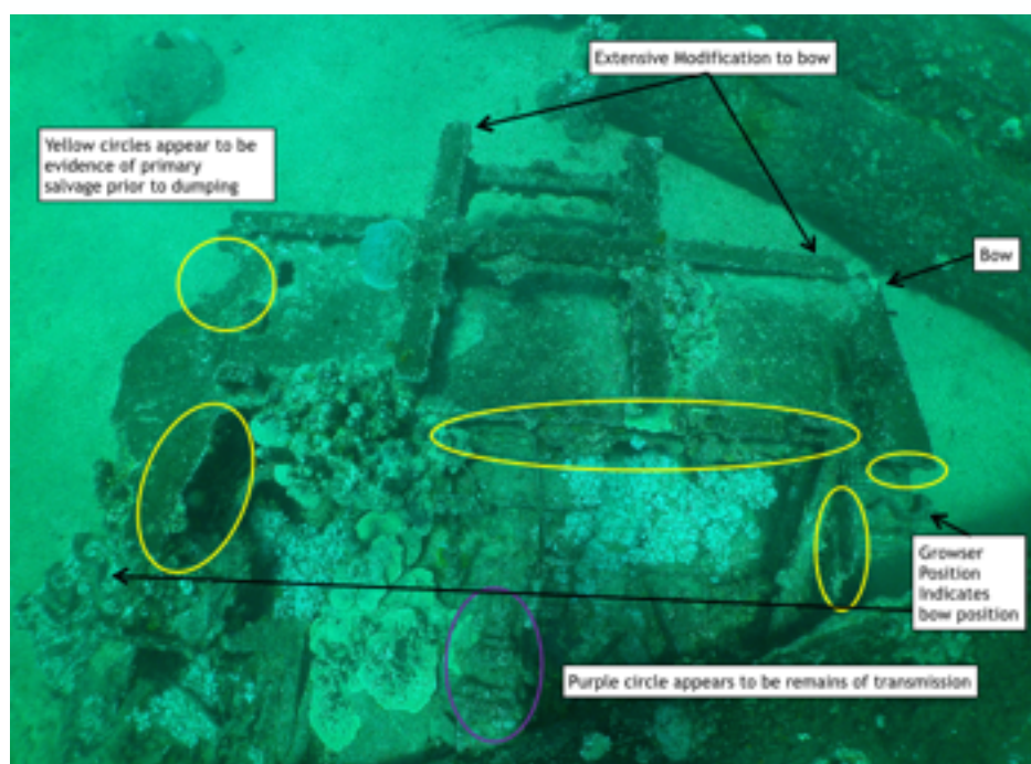
Figure 5. LVT examined for evidence of primary salvage prior to dumping at Seabee Junkyard (Arnold, 2014).
