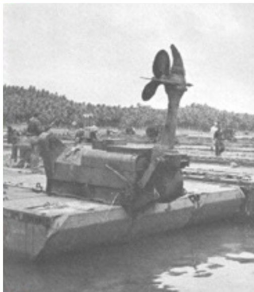
Figure 19. Raised pontoon outboard motor on a pontoon barge. Courtesy Jack Sprengle, U.S. Navy Seabee Museum, 2012.
