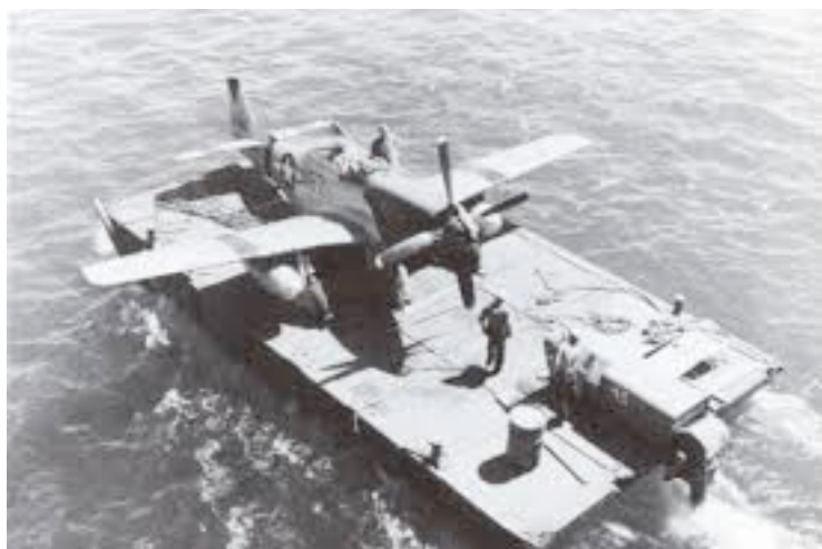
Figure 20. Pontoon barge, propelled by a pontoon outboard motor, transports a plane. Courtesy Jack Sprengle, U.S. Navy Seabee Museum, 2012.
